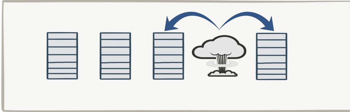
A 'replica' takes over on machine failure
